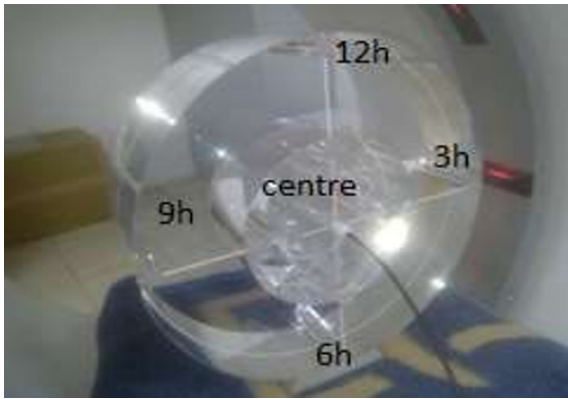
Fig. 5. CTDI100 measurement in PMMA body phantom. The phantom has been placed on the CT table with its long axis aligned with the gantry's axis of rotation. It has a diameter of 32 cm.
