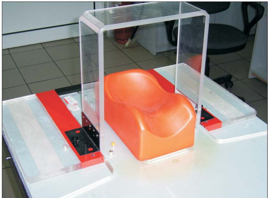
Phot. 1. Frame from perspex, fixed to the plate
