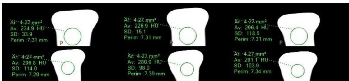
Figure 4: Measured Hounsfield Unit (HU) values of the fabricated epoxy-TiO 2 samples under clinical CT conditions
