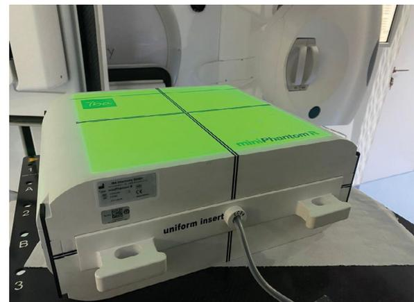
Fig. 14. Point dose measurement setup using CC04 Chamber
