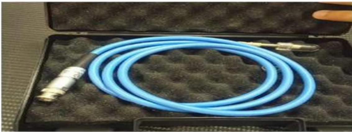
Fig. 4. The semi flex 3D PTW-31021 ionization chamber.
