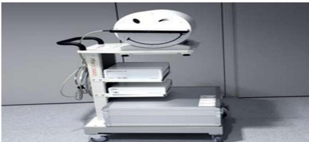
Fig. 5. The Octavius 4D phantom, with a 2D 1600 SRS matrix of liquid ionization chambers.
