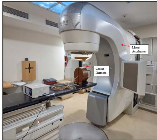
Fig. 2. Shows the Point dose measurement setup using Cheese Phantom along with A1SL chamber in Linear Accelerator
