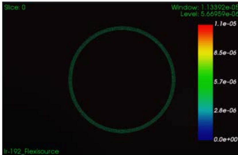
Fig. 1. Dose Distribution from simulation output generated by GATE: calculating S_k by placing a ring (dose actors) at 1 m from the source
