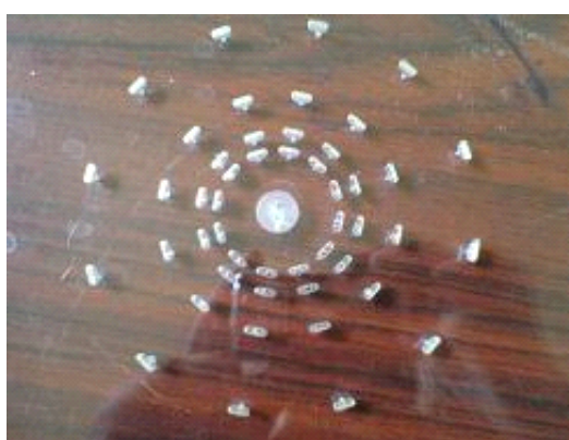
Fig. 5. The phantom used for the 125I source dosimetry
