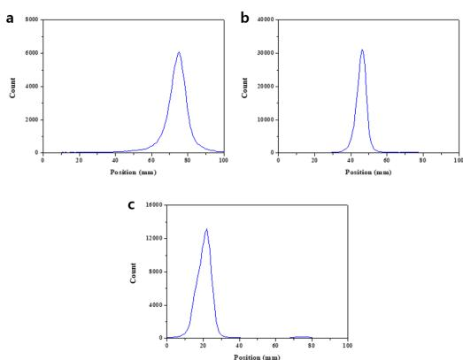
**Fig. 4.** Sc-44 labeling confirmation graph using ITLC. Free Sc-44 (a), Sc-44 labeled DOTA (b), and Sc-44 labeled DOTA-[Nle]-cCCK (c) were confirmed through ITLC. Peaks were formed at the following positions: 78 mm (a), 43 mm (b) and 21 mm (c).
